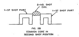
In this type of mold construction, for a one out tool there would be two identical cores, one first shot cavity and one last shot cavity. Basically this type of design will work whenever the main core side features can all be of first shot material or can readily be shut off on the first shot by steel from the cavity side. Again, this is more expensive than a core pull but is a fairly common concept and works very well.
