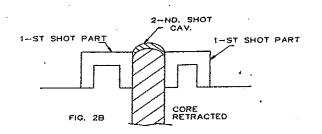
Figures 1A and 1B and Figures 2A and 2B show cross sections of such parts. The second shot cavity space is made available by the retraction of a core.
