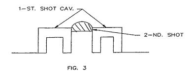
A core pull will not work without a part change. This part could be molded in an automatic rotating or indexing mold of common core design. However, this type of construction is considerably more expensive whether you use an automatic indexing mold base or a conventional mold base on a rotating platen style molding machine. In either case you require a larger base and twice as many cores and cavities, per part.
