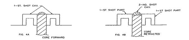
If the last shot contour could have a small flat of last shot material around it's periphery, without compromising the parts function, a core pull would work. The retractable core would seal against the flat and keep first shot material out of the last shot cavity.
