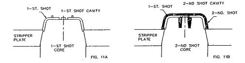
A stripper plate design is normally used only if there are first shot part features that can seal against the last shot cavity surface, such as graphics. This is needed to hold the first shot part in place, seated on the last shot core.
